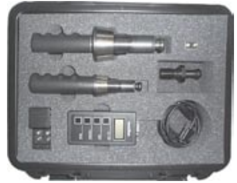
ForceCheck sets come complete with measuring bar, readout, connecting cable, NiMH rechargeable battery, charger, and a heavy-duty carrying case.
